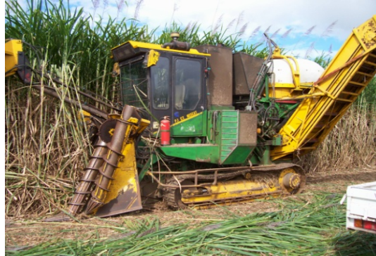
Typical track drive Cane Harvester
